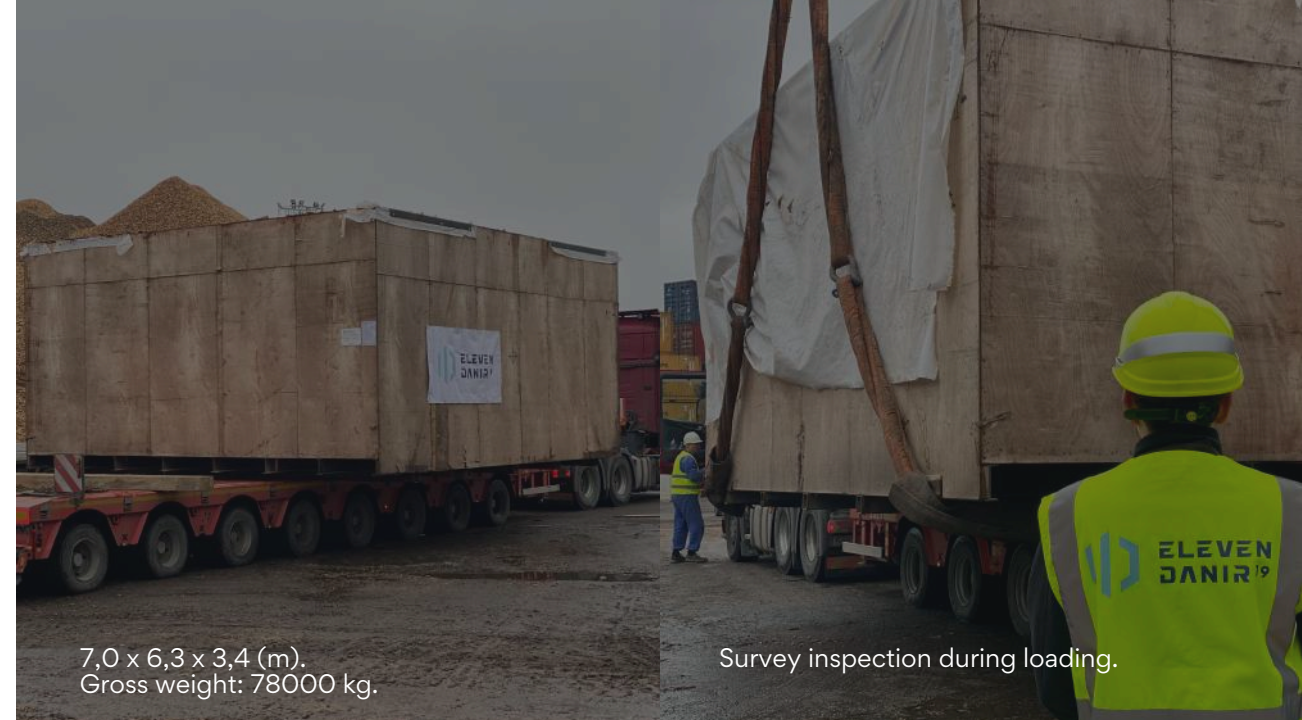
8 axles open trailer for out of gauge cargo.
